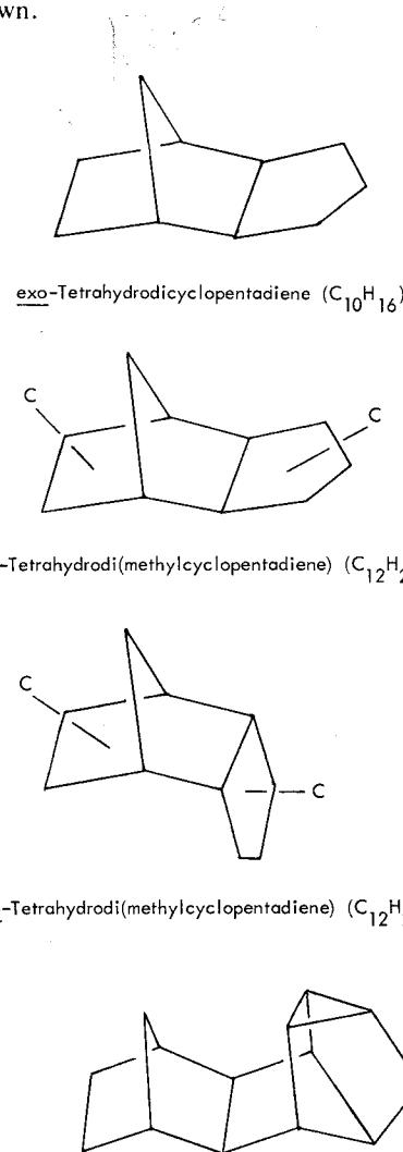
Fig. 1 Carbon skeletons of hydrocarbon fuels.
